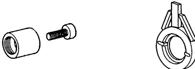
7. Remove the fixing nut of the rear bearing by means of the special key re. 180786 having previously moved it from the safety flange, to manage this operation, it is necessary a nylon hammer.
