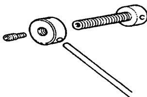
54. Remove the inserting tool and lubricate seal, with grease SHELL ALVANIA-3, located at the rear bearing and fix as convenient screws.
