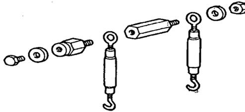
12. Remove screws that fix the bearing box and place the four extractor screws re. 146985.
