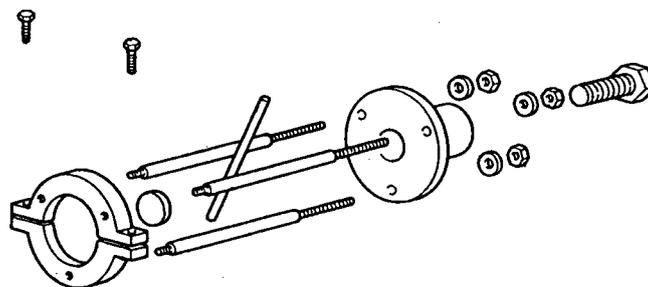
20. Remove the inner ring of the bearing by means of key re. 172007 and the handle re. 171967, for this operation alternately use wires re. 179341. At the same time, the toric gasket located at the bottom outer drum can be removed.
