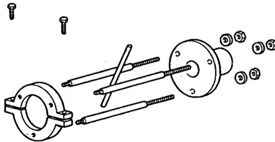
28. Lubricate screw re. 171439 (with bolt re. 171975 & nut re. 171447 assembled) and screw it to the shaft.
