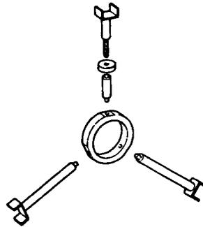
6. Remove basket pulley by means of the sleeve re. 180729-134981, having previously lifted the safety flange and removed the nut by means of key re. 180794, this sleeve is threaded to the pulley coupling and to unblock it tighten the screw re. 134981.
