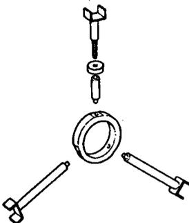
52. Place without screwing the plate of the rear bearing.
