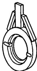
8. Remove the seal-holder cover of the rear bearing and replace the end ring.
