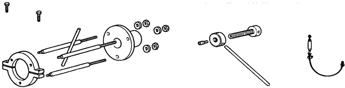
31. Disassemble the stainless steel plate which is screwed on the bearing box, and remove the aluminium platen that lodges the radial seal.
