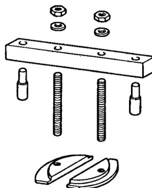
34. To remove the rear bearing use set re. 180620.
