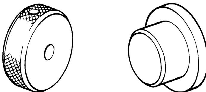
44.- Place suitably at the shaft the end ring together with adjustable washer by using the inserting tube re.194506 with complements re. 194514-194522 and bolt, washer and
